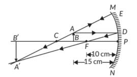
From ray diagram, v = -30 cm, i.e., beyond C Nature of image is real, inverted and magnified.
